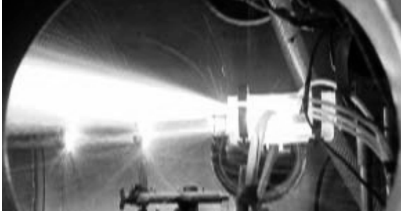
Fig. 21 Combustion of a supersonic ( M = 2 ) propane-airstream at use for ignition and burning stabilization, the combined microwave discharge created in aerodynamical channel with a rectangular cavity with angled rear wall at microwave pulse duration \tau = 10 \mu\text{s} , repetition frequency f = 100 \text{ Hz} , duration of dc current t = 1 \text{ s} , time exposure is 20 ms. The supersonic air–propane flow is directed from right to left.
